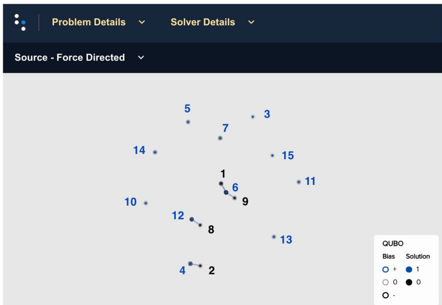
Fig. 6 Solution inspector in a D-Wave quantum annealer
